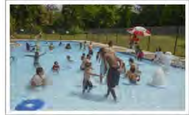
Zero entry pool with waterspray elements allows wheelchairs to enter directly into the water
